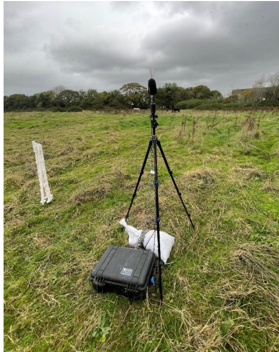
Figure 5: Noise Logger Setup
