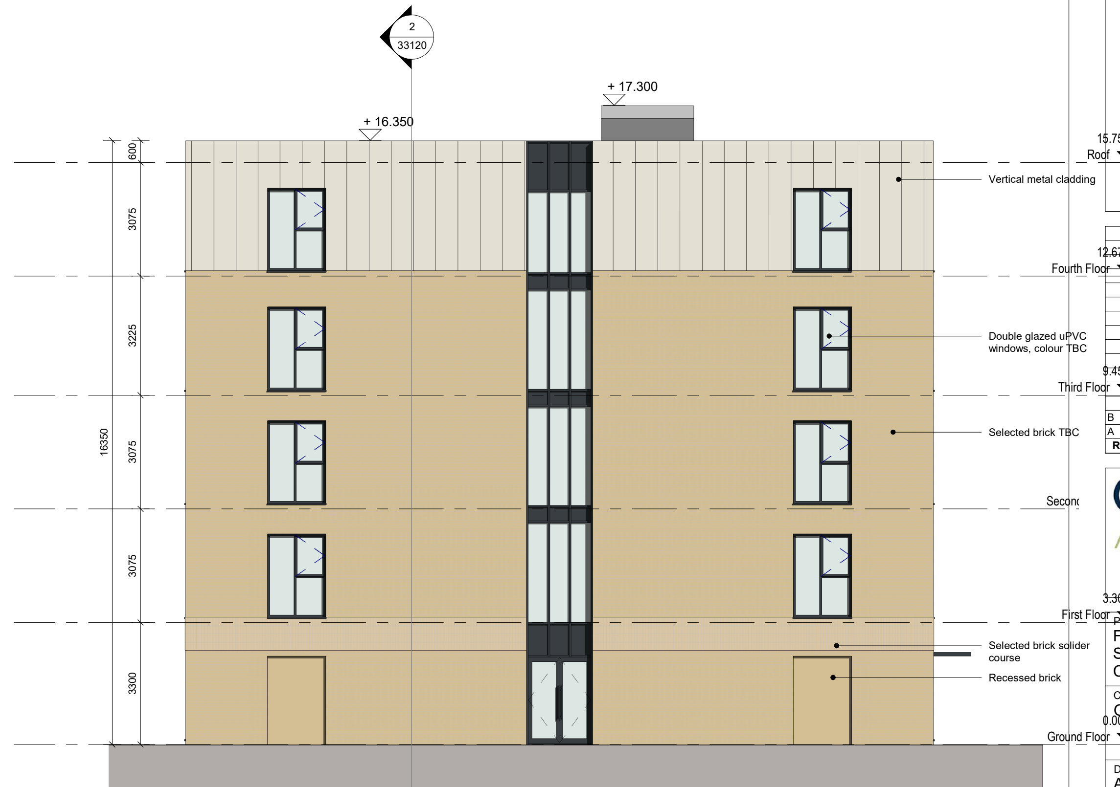
4 Apartment Block B - South Elevation 1 : 100
