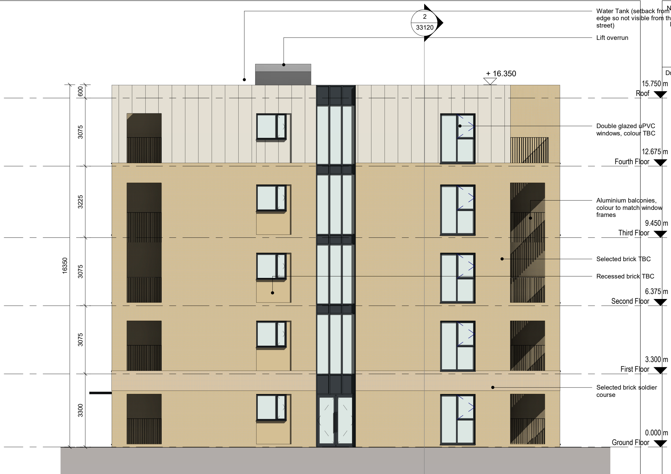
2 Apartment Block B - North Elevation 1 : 100
