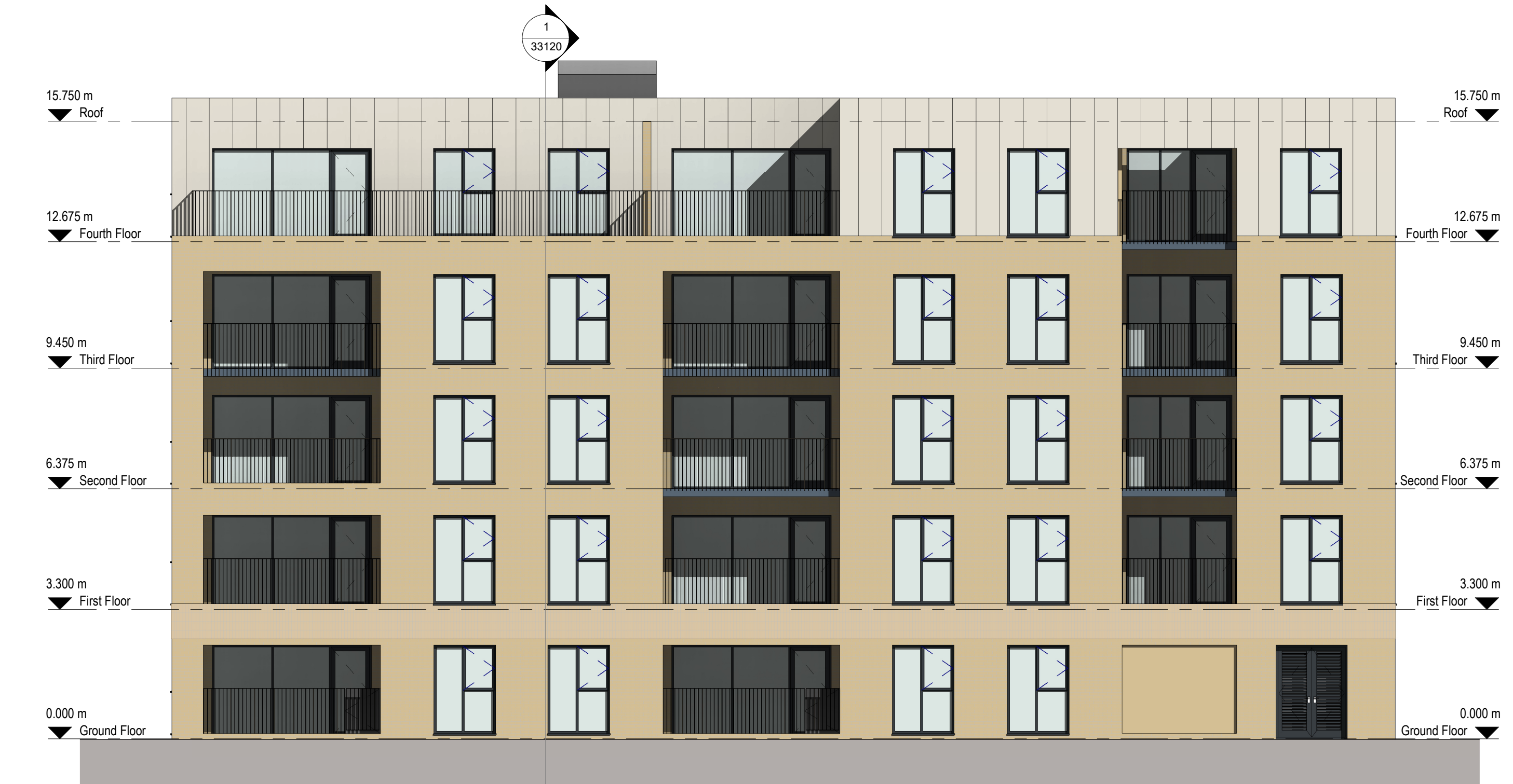
3 Apartment Block B - West Elevation 1 : 100
