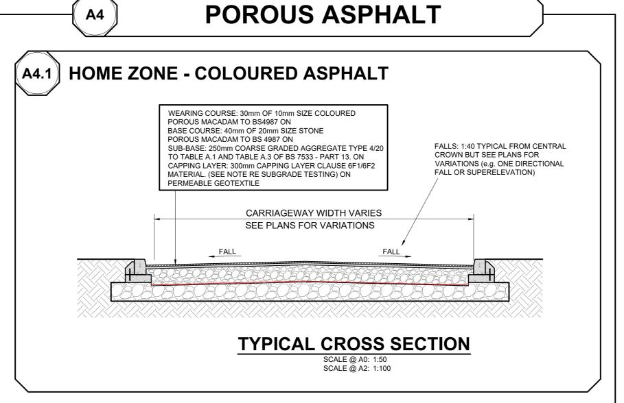
. EDGE OF EXISTING CARRIAGEWAY TO BE CUT BACK BY 0.5m WITH A ROTARY SAW TO FORM A VERTICAL FACE.
